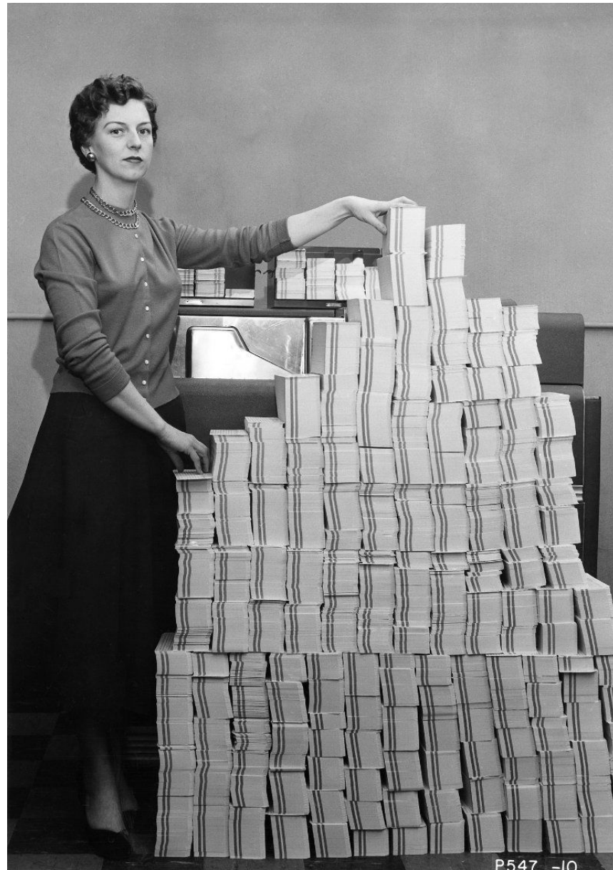
Stack of 62,500 punched cards 5 MB worth, holding the control program for the giant SAGE military computer network. 1955
