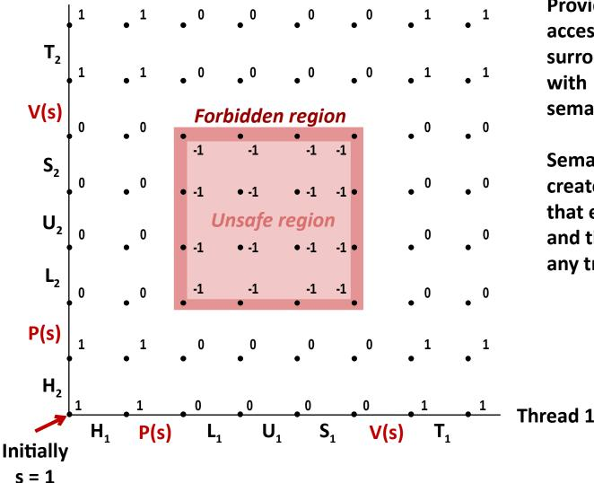
Provide mutually exclusive access to shared variable by surrounding critical section with *P* and *V* operations on semaphore s (initially set to 1)
