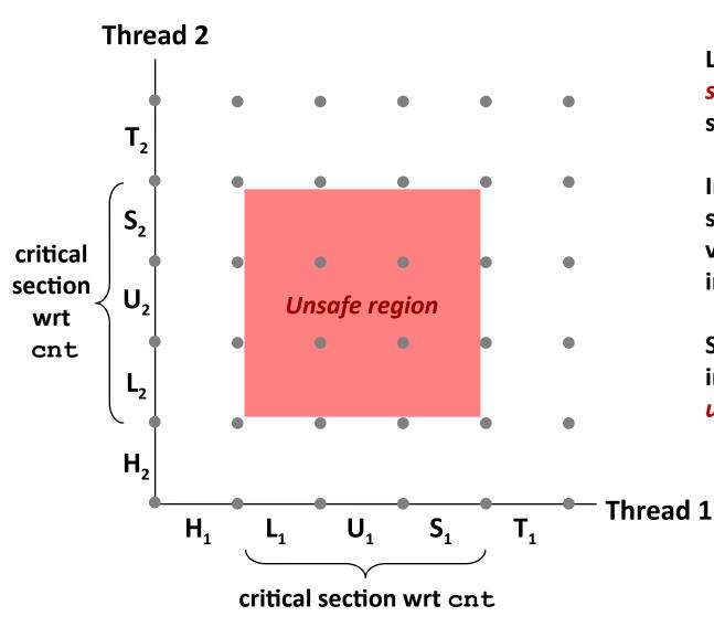
L, U, and S form a *critical section* with respect to the shared variable cnt
