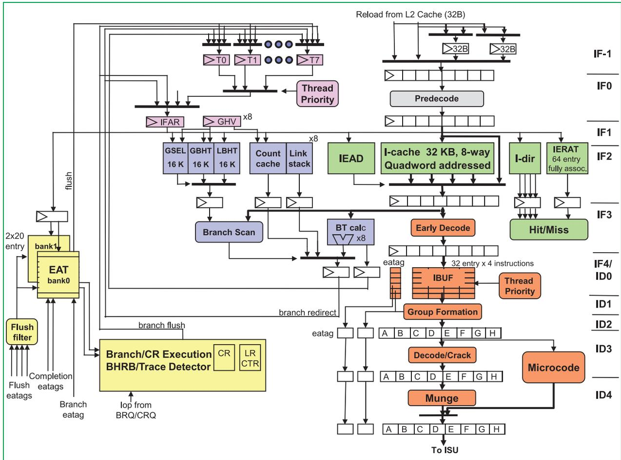
**Figure 3** POWER8 instruction fetch unit logical flow. The labels on the right of the figure denote the instruction fetch (IF) and instruction decode (ID) stages. (EAT: effective address table, eatag: effective address tag; iop: internal operation.)
