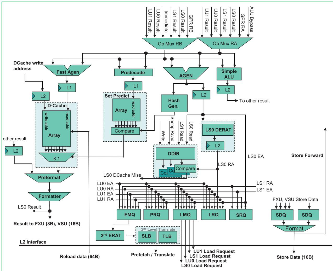
**Figure 6** POWER8 LSU micro architecture (LS0 pipe shown).
